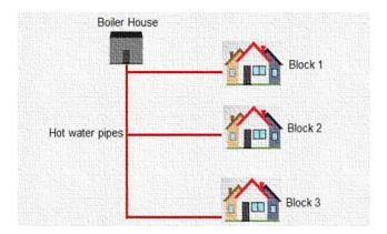
District heating properties are served from a main boiler house. These pump hot water into the radiators and cylinders in each property.
